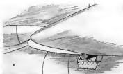
Mechanically connected to flap system, stabilizer is also flexed up from fixed slot position. Slaves great at front spar is also visible. Aileron connection is at rear spar for flap deflection of flap. Stabilizer moves 4 deg.
